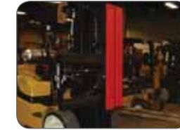
Sideshifting Fork Positioning Gypsum Handler
