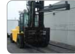
Sideshifting Fork Positioner with Load Hold-Down
